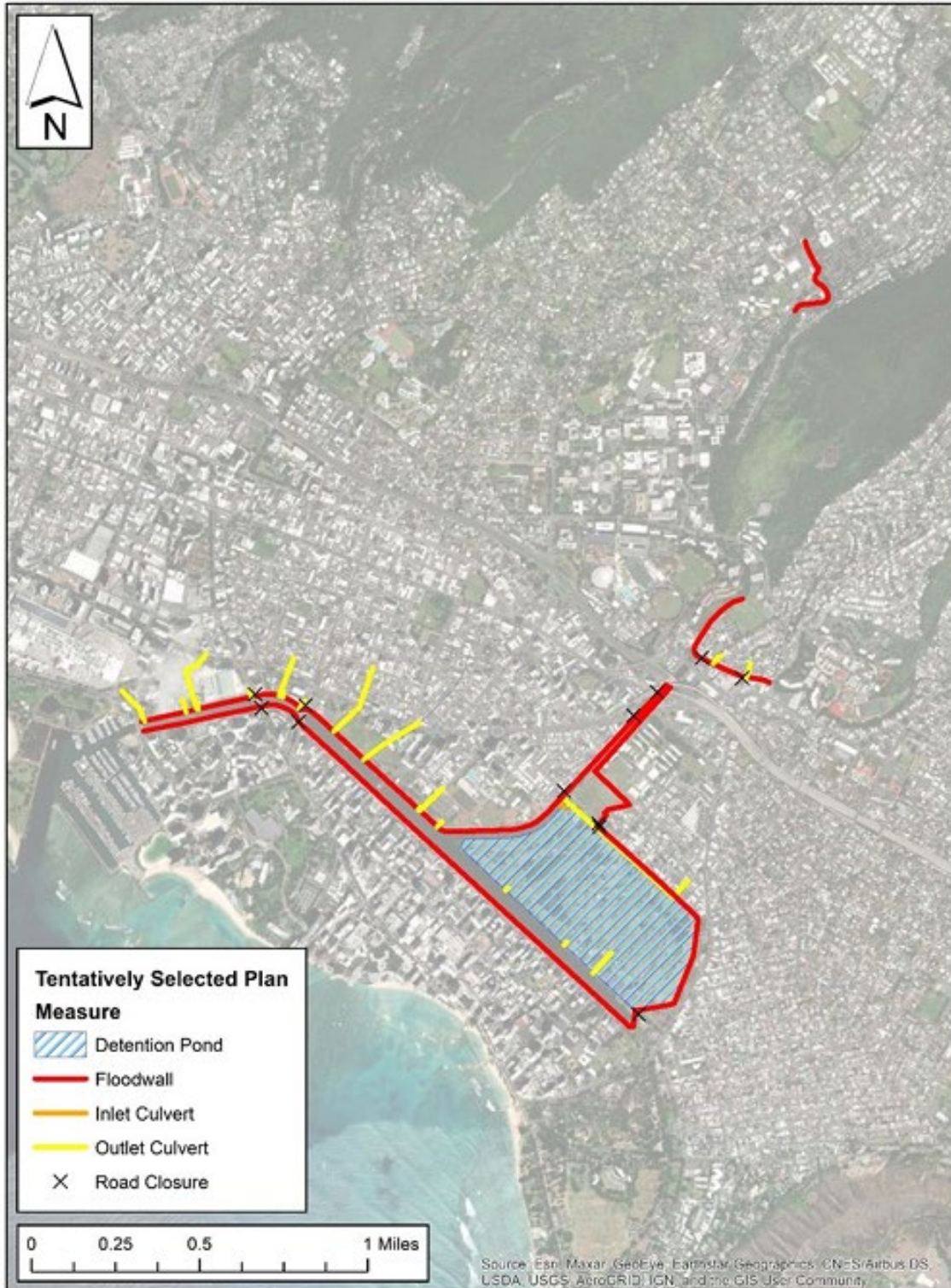
Figure 3. Conceptual diagram of proposed floodwall from Ala Wai Flood Risk Management Project (Alternative 5.1; US Army Corps of Engineers, 2023)
