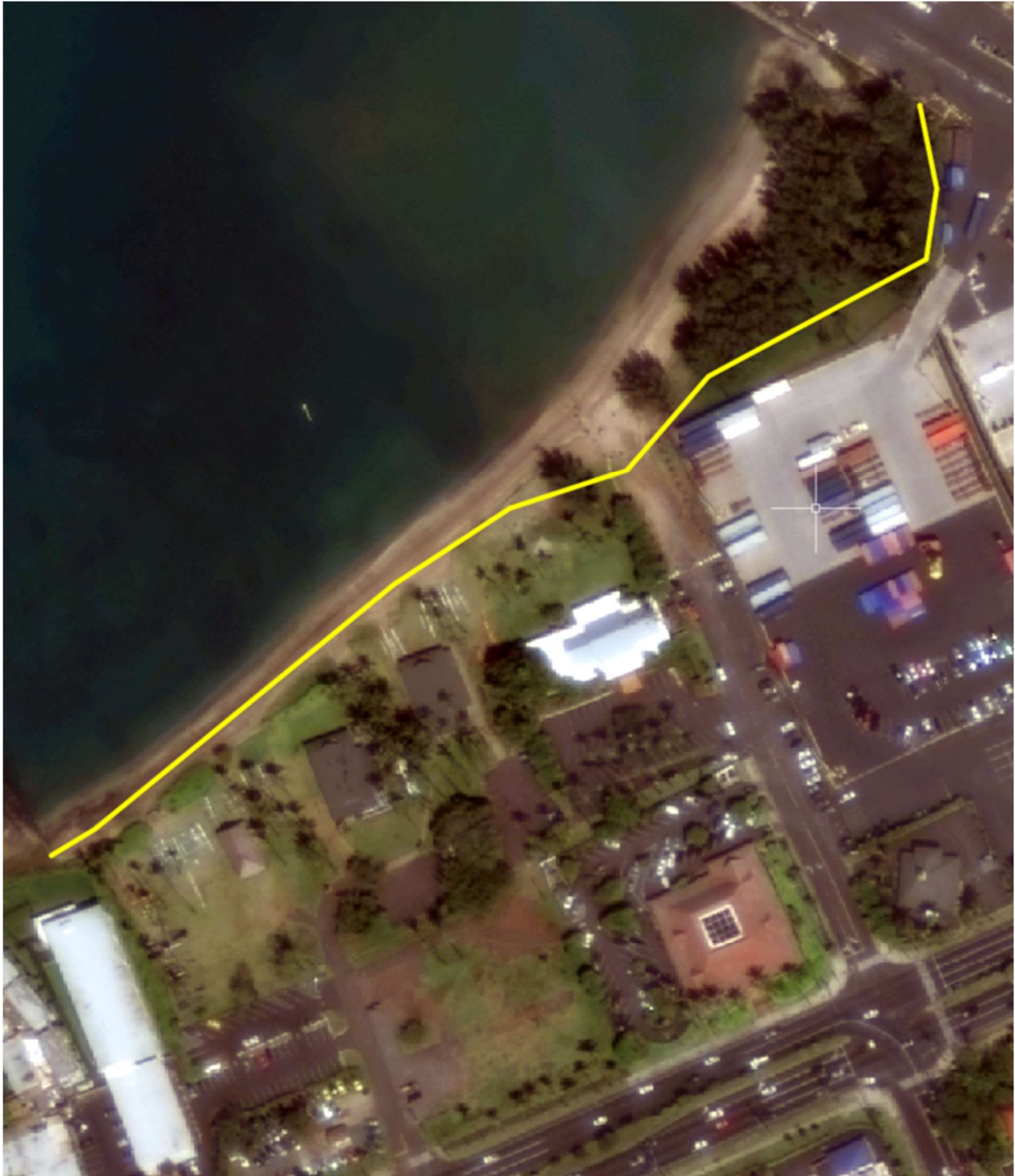
Figure13. A trace of the shoreline position in 1950 (yellow line) overlaid on an aerial photo from 2015, indicating accretion or fill has occurred along the northeast portion of the shoreline, while the southwest portion has been stable or eroded slightly.
