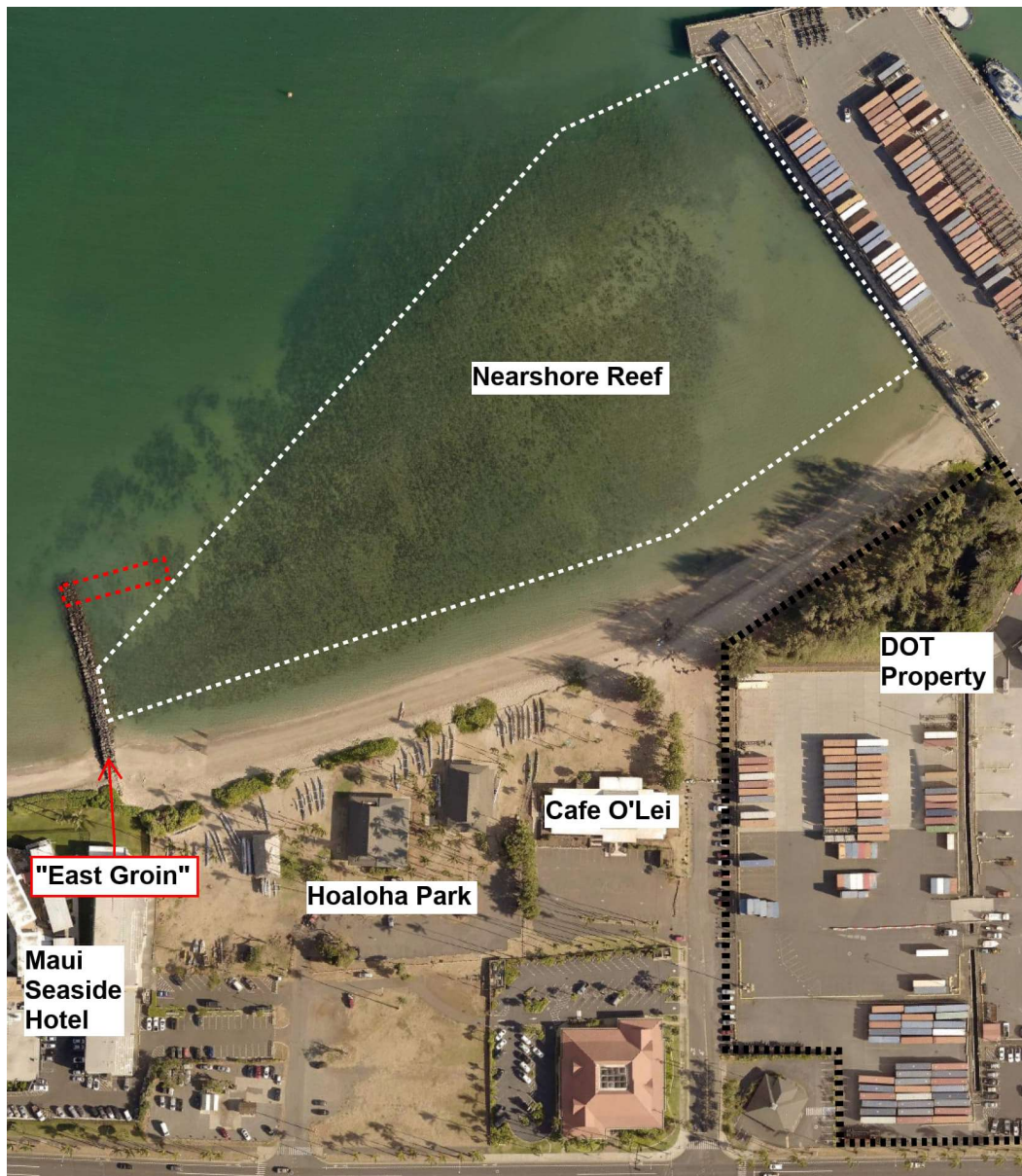
Figure 26. Aerial photograph of Hoaloha Park, with the nearshore reef area outlined in white, and a conceptual East Groin extension sketched in red.
